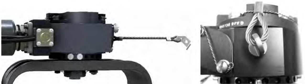
Figure 9 Safety Cable Attached to Gearbox
