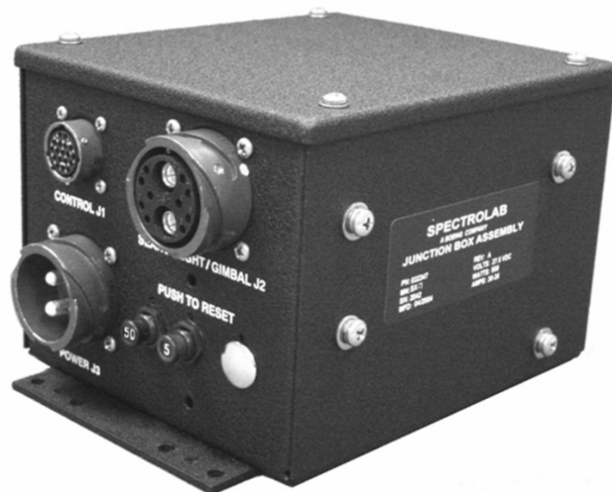
Figure 18 SX-7 Junction Box
